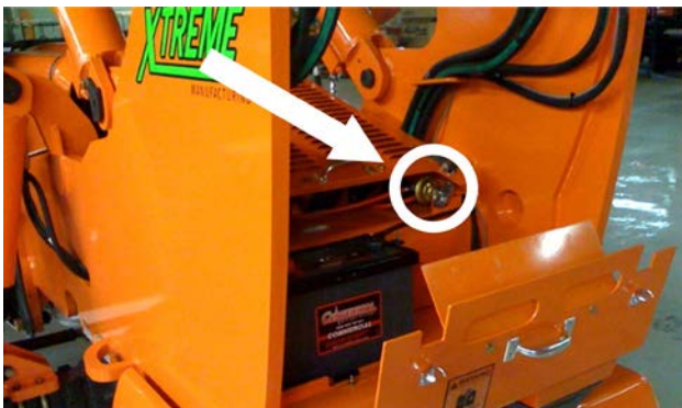
Figure 8-5. Battery Disconnect Switch.
