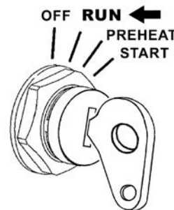
Figure 7-12. Ignition Switch Automatically Returns To RUN.
