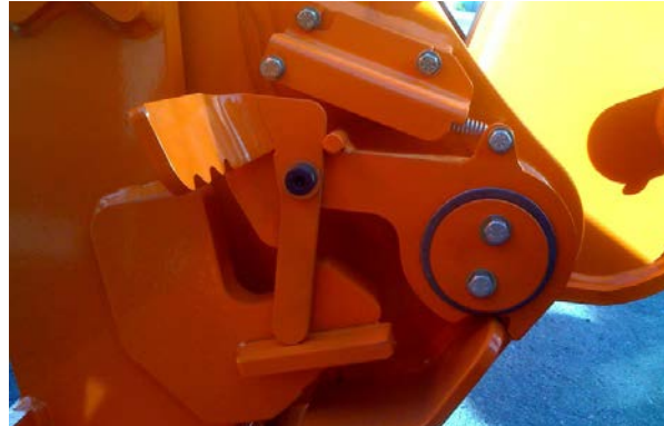
Figure 7-24. Ensure Latch Is Fully Open. This Position Is For Attachment Removal Only.
