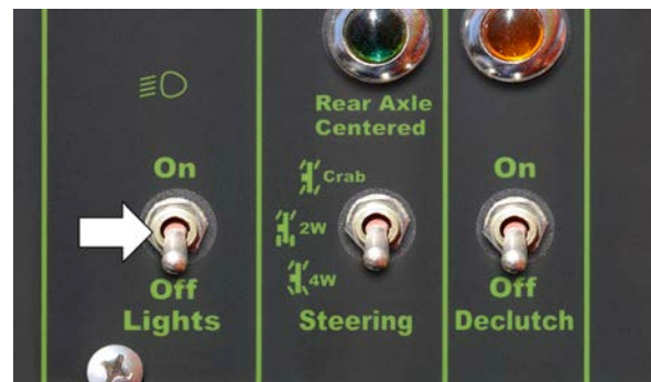
Figure 6-28. Work Light Switch.
