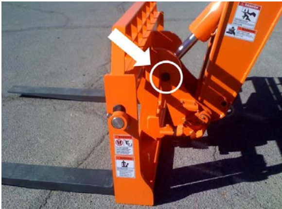
Figure 7-21. Drive Vehicle Forward To Align Pivot Pins With Attachment Hooks.
