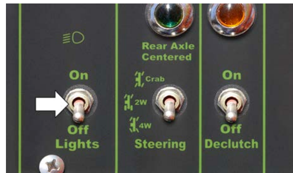
Figure 6-28. Work Light Switch.
