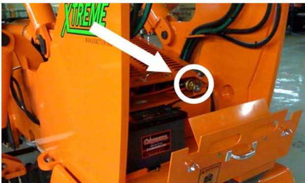
Figure 8-5. Battery Disconnect Switch.
