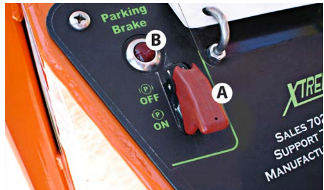
Figure 7-8. Parking Brake Switch (A) Must Be ON (Engaged) To Start The Reach Forklift.
